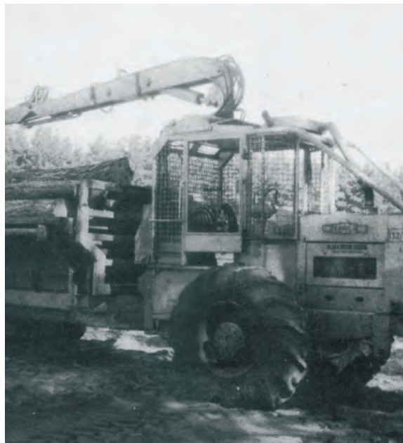
■ The Leyland Mammoth Major. Fully laden this vehicle with trailer can carry up to 10,000 super feet of log, the largest capacity being used in our Industry.
